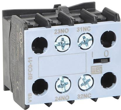
WEG Electric auxiliary contact, front mount, (1) N.O./ (1) N.C. contact(s), 6A @ 120 VAC/0.55A @ 120 VDC. For use with any 3-pole CWC07 through CWC016 series miniature contactor.
