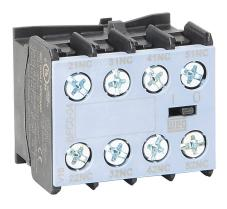
WEG Electric auxiliary contact, front mount, (4) N.C. contact(s), 6A @ 120 VAC/0.55A @ 120 VDC. For use with any 3-pole CWC07 through CWC016 series miniature contactor with standard consumption AC or DC coils.
