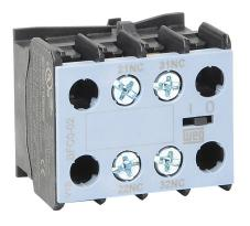
WEG Electric auxiliary contact, front mount, (2) N.C. contact(s), 6A @ 120 VAC/0.55A @ 120 VDC. For use with any 3-pole CWC07 through CWC016 series miniature contactor.
