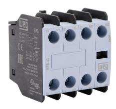
WEG Electric field installable auxiliary contact, front mount, (4) N.O. contact(s), 6A @ 120 VAC/0.22A @ 120 VDC, screw terminal. For use with CWB9 to CWB125 series contactors.
