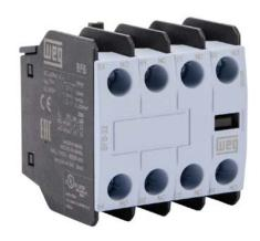
WEG Electric field installable auxiliary contact, front mount, (2) N.O./(2) N.C. contact(s), 6A @ 120 VAC/0.22A @ 120 VDC, screw terminal. For use with CWB9 to CWB125 series contactors.
