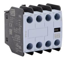
WEG Electric field installable auxiliary contact, front mount, (2) N.O./(2) N.C. contact(s), 6A @ 120 VAC/0.22A @ 120 VDC, screw terminal. For use with CWB9 to CWB125 series contactors.
