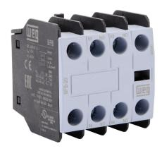
WEG Electric field installable auxiliary contact, front mount, (2) N.O. contact(s), 6A @ 120 VAC/0.22A @ 120 VDC, screw terminal. For use with CWB9 to CWB125 series contactors.
