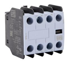
WEG Electric field installable auxiliary contact, front mount, (1) N.O./(1) N.C. contact(s), 6A @ 120 VAC/0.22A @ 120 VDC, screw terminal. For use with CWB9 to CWB125 series contactors.
