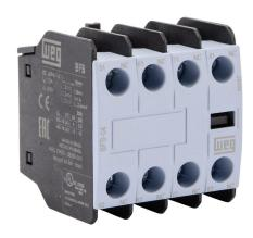
WEG Electric field installable auxiliary contact, front mount, (4) N.C. contact(s), 6A @ 120 VAC/0.22A @ 120 VDC, screw terminal. For use with CWB9 to CWB125 series contactors.
