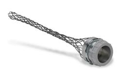
Bryant dust-tight strain relief grip, accepts cable diameter size 0.97 to 1.25in, 1-1/4in NPS male thread fitting, galvanized steel mesh, 9in length, indoor applications only. Steel locknut and insulating bushing included.
