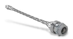
Bryant dust-tight strain relief grip, accepts cable diameter size 0.54 to 0.73in, 3/4in NPS male thread fitting, galvanized steel mesh, 6.5in length, indoor applications only. Steel locknut and insulating bushing included.
