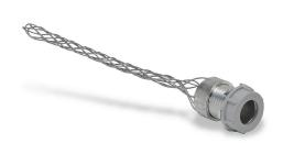
Bryant dust-tight strain relief grip, accepts cable diameter size 0.43 to 0.54in, 1/2in NPS male thread fitting, galvanized steel mesh, 4.75in length, indoor applications only. Steel locknut and insulating bushing included.
