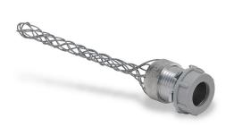
Bryant dust-tight strain relief grip, accepts cable diameter size 0.32 to 0.43in, 1/2in NPS male thread fitting, galvanized steel mesh, 3.75in length, indoor applications only. Steel locknut and insulating bushing included.
