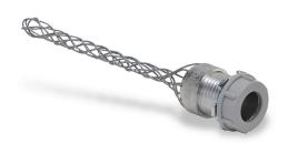
Bryant dust-tight strain relief grip, accepts cable diameter size 0.32 to 0.43in, 1/2in NPS male thread fitting, galvanized steel mesh, 3.75in length, indoor applications only. Steel locknut and insulating bushing included.
