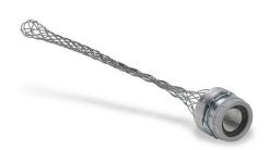
Bryant dust-tight strain relief grip, accepts cable diameter size 1.5 to 1.7in, 2in NPT male thread fitting, galvanized steel mesh, 13.25in length, indoor applications only. Steel locknut and insulating bushing included.
