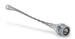
Bryant dust-tight strain relief grip, accepts cable diameter size 1.25 to 1.5in, 1-1/2in NPT male thread fitting, galvanized steel mesh, 11.75in length, indoor applications only. Steel locknut and insulating bushing included.
