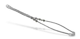
Bryant bus drop support grip, accepts cable diameter size 0.85 to 1in, closed, galvanized steel mesh, 8in length, single, eye length 8in, indoor applications only. For use with safety springs S40 or S80 to further reduce tension.
