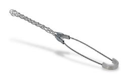
Bryant bus drop support grip, accepts cable diameter size 0.32 to 0.43in, closed, galvanized steel mesh, 4in length, single, eye length 4in, indoor applications only. For use with safety springs S40 or S80 to further reduce tension.
