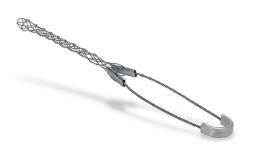
Bryant bus drop support grip, accepts cable diameter size 0.32 to 0.43in, closed, galvanized steel mesh, 4in length, single, eye length 4in, indoor applications only. For use with safety springs S40 or S80 to further reduce tension.
