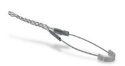
Bryant bus drop support grip, accepts cable diameter size 0.24 to 0.32in, closed, galvanized steel mesh, 3.5in length, single, eye length 3in, indoor applications only. For use with safety springs S40 or S80 to further reduce tension.
