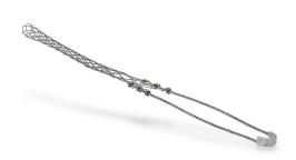
Bryant bus drop support grip, accepts cable diameter size 1 to 1.25in, closed, galvanized steel mesh, 9.5in length, single, eye length 9in, indoor applications only. For use with safety springs S40 or S80 to further reduce tension.
