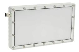
Lumher BD machine vision lighting, backlight, white light emission, 5000K, plus or minus 30 degrees,  $100 \times 190$ mm luminous field, continuous and strobe,  $125 \times 215 \times 25$ mm housing, 22.8-25.2 VDC operating voltage.
