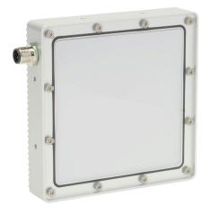
Lumher BD machine vision lighting, backlight, white light emission, 5000K, plus or minus 30 degrees, 100 x 100mm luminous field, continuous and strobe, 125 x 125 x 25mm housing, 22.8-25.2 VDC operating voltage.
