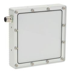
Lumher BD machine vision lighting, backlight, white light emission, 5000K, plus or minus 30 degrees,  $100 \times 100$ mm luminous field, continuous,  $125 \times 125 \times 25$ mm housing, 22.8-25.2 VDC operating voltage.
