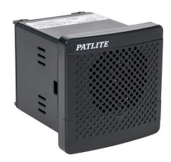
Patlite audible alarm, 90 dB at 1m, 191 Hz to 1.7 kHz tone frequency, (32) selectable tone(s), 12-24 VDC, panel or surface mount, ABS plastic housing, dark gray, IP54.
