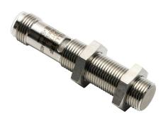
Balluff capacitive proximity sensor, tubular, 12mm diameter x 60mm body, stainless steel housing, NPN/PNP, N.C., 5mm sensing distance, flush, 100 Hz switching frequency, IP67, 4-pin M12 quick-disconnect.
