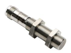
Balluff capacitive proximity sensor, tubular, 12mm diameter x 60mm body, stainless steel housing, NPN/PNP, N.O., 5mm sensing distance, flush, 100 Hz switching frequency, IP67, 4-pin M12 quick-disconnect.
