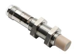
Balluff capacitive proximity sensor, tubular, 12mm diameter x 60mm body, stainless steel housing, NPN/PNP, N.C., 8mm sensing distance, non-flush, 100 Hz switching frequency, IP67, 4-pin M12 quick-disconnect.
