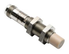
Balluff capacitive proximity sensor, tubular, 12mm diameter x 60mm body, stainless steel housing, NPN/PNP, N.O., 8mm sensing distance, non-flush, 100 Hz switching frequency, IP67, 4-pin M12 quick-disconnect.
