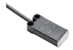
Balluff capacitive proximity sensor, rectangular, 34 x 16 x 8mm body, polypropylene (PP) housing, top sensing, PNP, N.O., 8mm sensing distance, flush, 100 Hz switching frequency, IP67, 4-pin M8 quick-disconnect.
