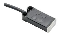
Balluff capacitive proximity sensor, rectangular, 34 x 16 x 8mm body, polypropylene (PP) housing, top sensing, PNP, N.O., 8mm sensing distance, flush, 50 Hz switching frequency, IP67, pigtail.
