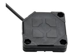
Balluff capacitive proximity sensor, rectangular, 40 x 40 x 10mm body, polybutylene terephthalate housing, top sensing, PNP, N.O., 20mm sensing distance, flush, 100 Hz switching frequency, IP67, 3-pin M8 quick-disconnect.
