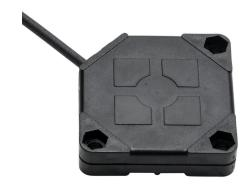
Balluff capacitive proximity sensor, rectangular, 40 x 40 x 10mm body, polybutylene terephthalate housing, top sensing, NPN/PNP, N.O./N.C. selectable, 20mm sensing distance, flush, 100 Hz switching frequency, IP67, pigtail.
