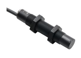
Balluff capacitive proximity sensor, tubular, 12mm diameter x 61mm body, polybutylene terephthalate housing, PNP, N.C., 8mm sensing distance, non-flush, 100 Hz switching frequency, IP67, pigtail.
