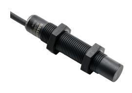
Balluff capacitive proximity sensor, tubular, 12mm diameter x 61mm body, polybutylene terephthalate housing, PNP, N.O., 8mm sensing distance, non-flush, 100 Hz switching frequency, IP67, pigtail.
