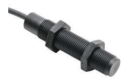
Balluff capacitive proximity sensor, tubular, 12mm diameter x 61mm body, polybutylene terephthalate housing, PNP, N.O., 4mm sensing distance, flush, 100 Hz switching frequency, IP67, pigtail.
