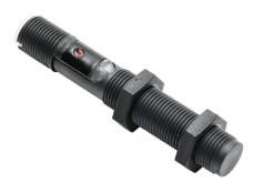
Balluff capacitive proximity sensor, tubular, 12mm diameter x 75mm body, polybutylene terephthalate housing, PNP, N.O., 4mm sensing distance, flush, 100 Hz switching frequency, IP67, 4-pin M12 quick-disconnect.
