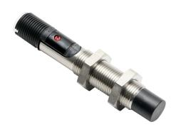
Balluff capacitive proximity sensor, tubular, 12mm diameter x 75mm body, stainless steel housing, PNP, N.O., 8mm sensing distance, non-flush, 100 Hz switching frequency, IP67, 4-pin M12 quick-disconnect.
