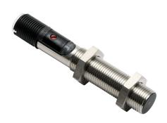
Balluff capacitive proximity sensor, tubular, 12mm diameter x 75mm body, stainless steel housing, PNP, N.C., 4mm sensing distance, flush, 100 Hz switching frequency, IP67, 4-pin M12 quick-disconnect.
