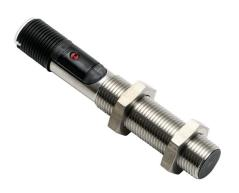
Balluff capacitive proximity sensor, tubular, 12mm diameter x 75mm body, stainless steel housing, PNP, N.O., 4mm sensing distance, flush, 100 Hz switching frequency, IP67, 4-pin M12 quick-disconnect.
