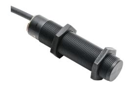
Balluff capacitive proximity sensor, tubular, 18mm diameter x 75mm body, polybutylene terephthalate housing, PNP, N.O., 8mm sensing distance, flush, 100 Hz switching frequency, IP67, pigtail.
