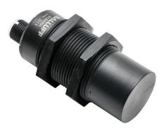
Balluff capacitive proximity sensor, tubular, 30mm diameter x 78.5mm body, polybutylene terephthalate housing, PNP, N.O., 25mm sensing distance, non-flush, 100 Hz switching frequency, IP67, 4-pin M12 quick-disconnect.
