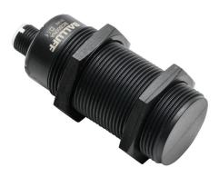
Balluff capacitive proximity sensor, tubular, 30mm diameter x 79mm body, polybutylene terephthalate housing, PNP, N.O., 15mm sensing distance, flush, 100 Hz switching frequency, IP67, 4-pin M12 quick-disconnect.
