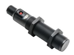
Balluff capacitive proximity sensor, tubular, 18mm diameter x 88.5mm body, polybutylene terephthalate housing, NPN, N.O., 8mm sensing distance, flush, 100 Hz switching frequency, IP67, 4-pin M12 quick-disconnect.
