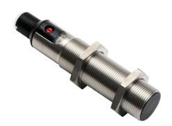
Balluff capacitive proximity sensor, tubular, 18mm diameter x 88.5mm body, stainless steel housing, PNP, N.O., 8mm sensing distance, flush, 100 Hz switching frequency, IP67, 4-pin M12 quick-disconnect.
