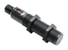
Balluff capacitive proximity sensor, tubular, 18mm diameter x 88.5mm body, polybutylene terephthalate housing, PNP, N.O., 8mm sensing distance, flush, 100 Hz switching frequency, IP67, 4-pin M12 quick-disconnect.
