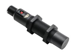
Balluff capacitive proximity sensor, tubular, 18mm diameter x 88.5mm body, polybutylene terephthalate housing, PNP, N.O., 15mm sensing distance, non-flush, 100 Hz switching frequency, IP67, 4-pin M12 quick-disconnect.
