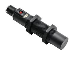
Balluff capacitive proximity sensor, tubular, 18mm diameter x 88.5mm body, polybutylene terephthalate housing, PNP, N.O., 15mm sensing distance, non-flush, 100 Hz switching frequency, IP67, 4-pin M12 quick-disconnect.
