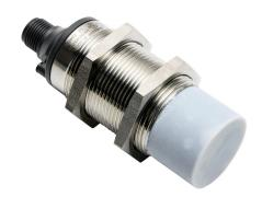
Balluff capacitive proximity sensor, tubular, 30mm diameter x 86.5mm body, stainless steel housing, PNP, N.O./N.C. selectable, 30mm sensing distance, non-flush, 100 Hz switching frequency, IP66, 4-pin M12 quick-disconnect.
