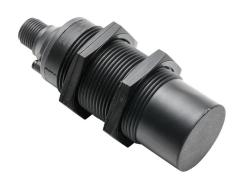
Balluff capacitive proximity sensor, tubular, 30mm diameter x 87mm body, polybutylene terephthalate housing, PNP, N.O./N.C. selectable, 30mm sensing distance, non-flush, 100 Hz switching frequency, IP66, 4-pin M12 quick-disconnect.
