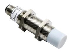
Balluff capacitive proximity sensor, tubular, 18mm diameter x 75mm body, stainless steel housing, PNP, N.O., 15mm sensing distance, non-flush, 100 Hz switching frequency, IP67, 4-pin M12 quick-disconnect.
