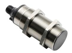
Balluff capacitive proximity sensor, tubular, 30mm diameter x 87mm body, stainless steel housing, PNP, N.O./N.C. selectable, 20mm sensing distance, flush, 100 Hz switching frequency, IP66, 4-pin M12 quick-disconnect.
