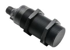
Balluff capacitive proximity sensor, tubular, 30mm diameter x 87mm body, polybutylene terephthalate housing, PNP, N.O./N.C. selectable, 20mm sensing distance, flush, 100 Hz switching frequency, IP66, 4-pin M12 quick-disconnect.
