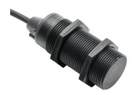
Balluff capacitive proximity sensor, tubular, 30mm diameter x 82mm body, polybutylene terephthalate housing, PNP, N.O./N.C. selectable, 20mm sensing distance, flush, 100 Hz switching frequency, IP66, pigtail.
